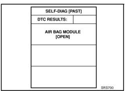
If no malfunction is detected on "SELF-DIAG [PAST]", touch "BACK" and go back to "SELECT DIAG MODE".
