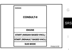
Touch "AIR BAG". If "AIR BAG" is not indicated, refer to GI-40, "CONSULT-II Data Link Connector (DLC) Circuit".
