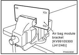
2. Match the hole in air bag module bracket (held in vise) and front passenger air bag module and fix them with one bolt [M8  $\times$  25 - 30 mm (0.98 - 1.18 in)].
