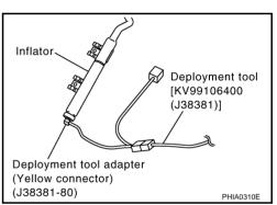
3. Put the inflator connected with the deployment tool [SST: KV99106400 (J38381)] into a tire without a wheel.
