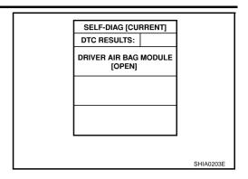
If no malfunction is detected on "SELF-DIAG [CURRENT]" even though malfunction is detected in "SRS Operation Check", check the battery voltage. If the battery voltage is less than 9V, charge or replace the battery. Then go to <u>SRS-23</u>, "<u>DIAGNOSTIC PROCEDURE 3</u>". If the battery voltage is OK, go to <u>SRS-25</u>, "<u>DIAGNOSTIC PROCEDURE 4</u> (<u>CONTINUED FROM DIAGNOSTIC PROCEDURE 2</u>)" to diagnose the following cases:
