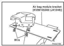
4. Connect deployment tool adapter (SST: J38381-80) to air bag module connector and deployment tool connector [SST: KV9910400 (J38381)].
