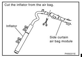
2. Connect deployment tool [SST: KV99106400 (J38381)] and deployment tool adapter yellow connector (SST: J38381-80) to the inflator.
